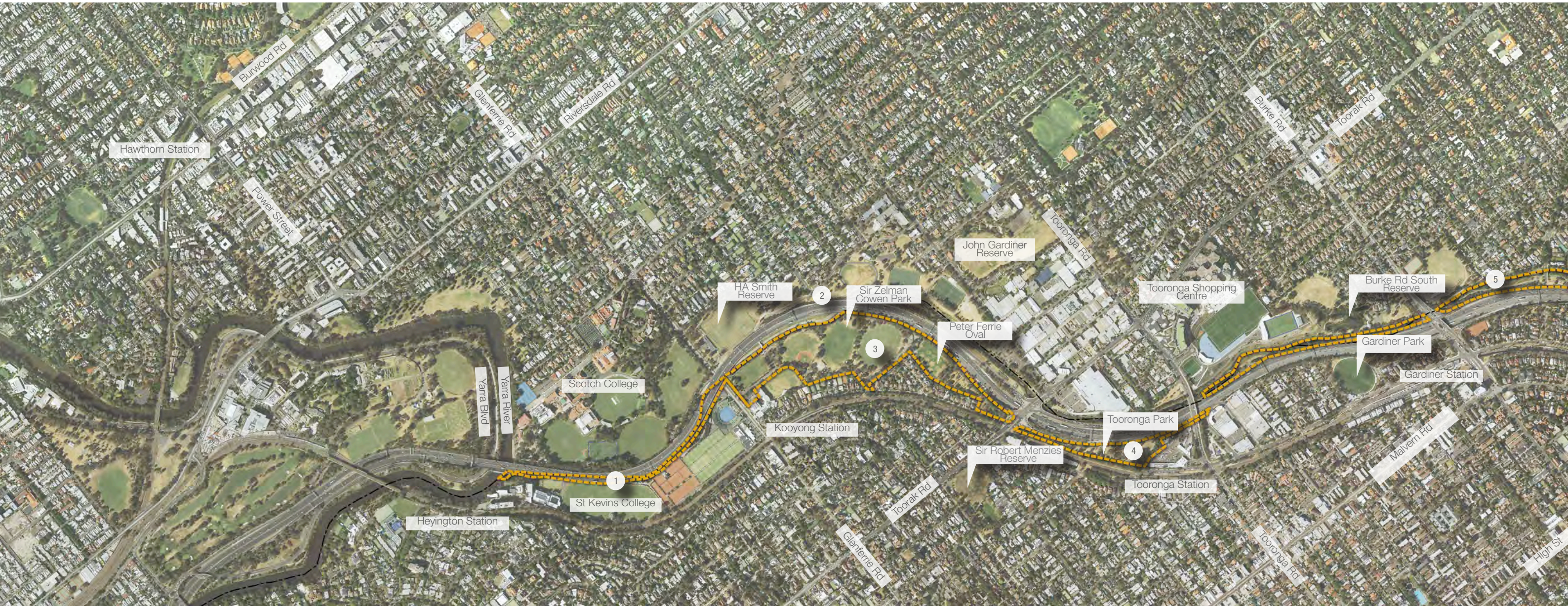
2 Concrete Lined Gardiners Creek (KooyongKoot) Highly modified and urbanised creek, to facilitate water management for the catchment. Sections of the creek were lined with concrete to increase water capacity.
