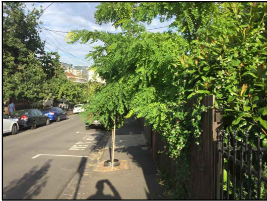
1. TRIM VEGETATION TO MAXIMISE EFFECTIVE FOOTPATH WIDTH. IMPROVE FOOTPATH PAVEMENT ALONG ROUTE TO ADDRESS UNEVEN SURFACES
