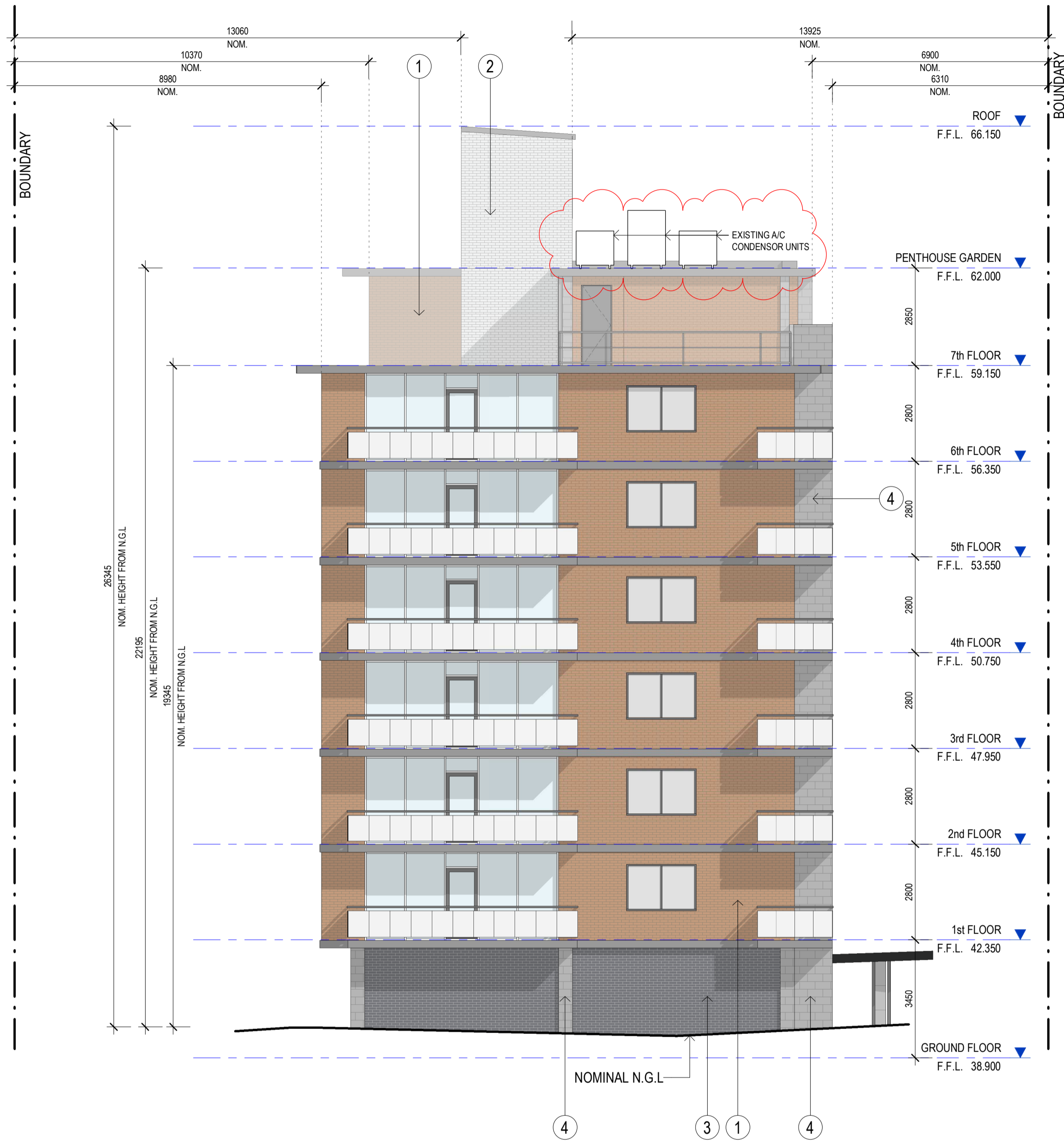
SOUTH ELEVATION - EXISTING SCALE: 1 : 100
