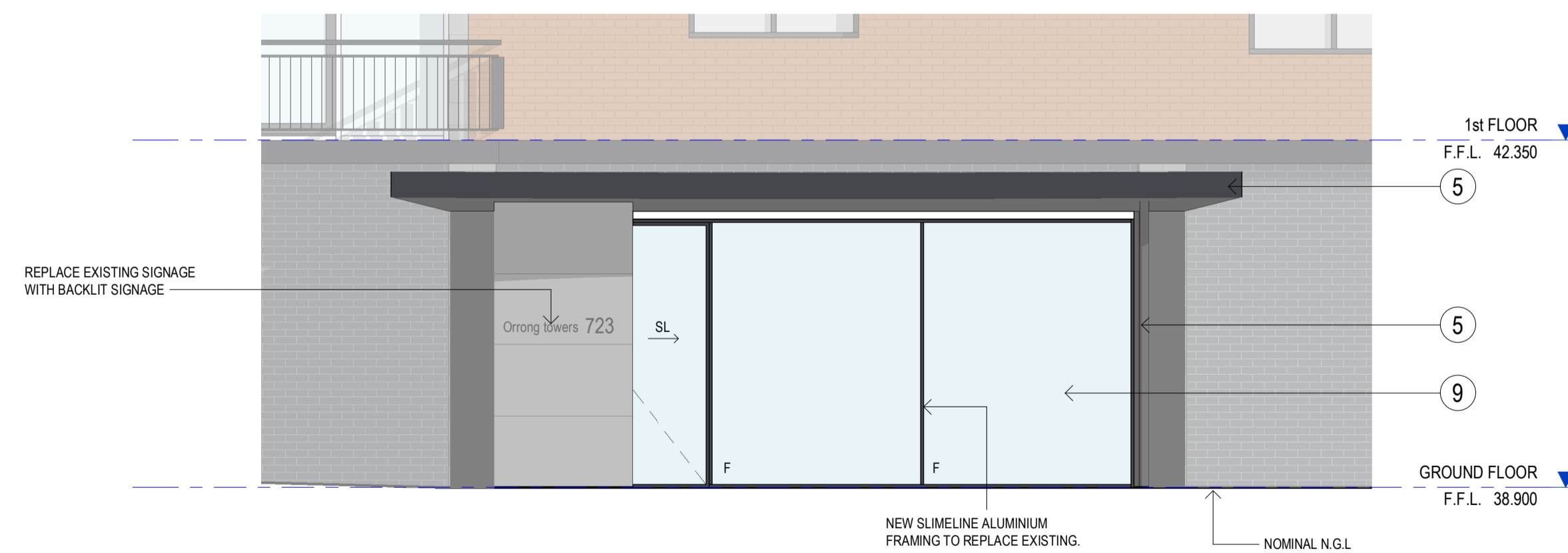
2 PROPOSED MAIN ENTRY UPGRADE WORKS SCALE: 1 : 50
