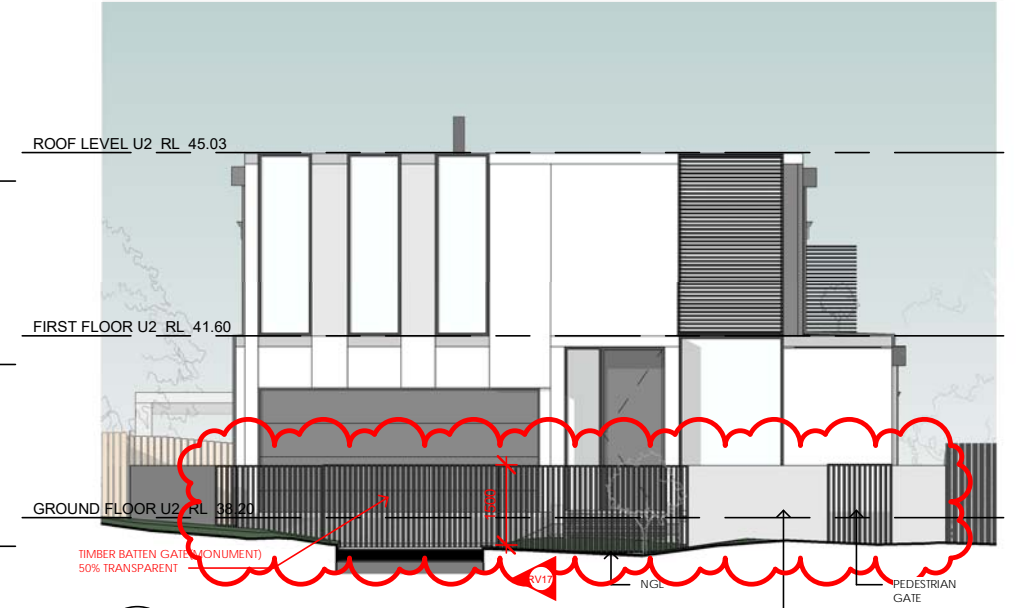
6 NORTH ELEVATION - UNIT 2 WITH FENCE Scale 1 : 100
