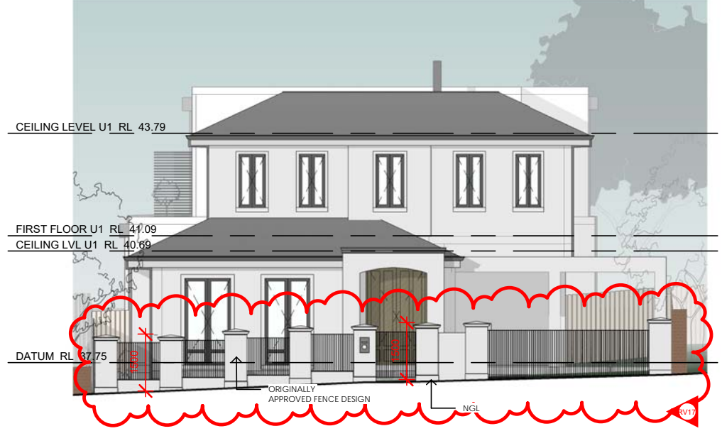
5 SOUTH ELEVATION - UNIT 1 WITH FENCE Scale 1 : 100
