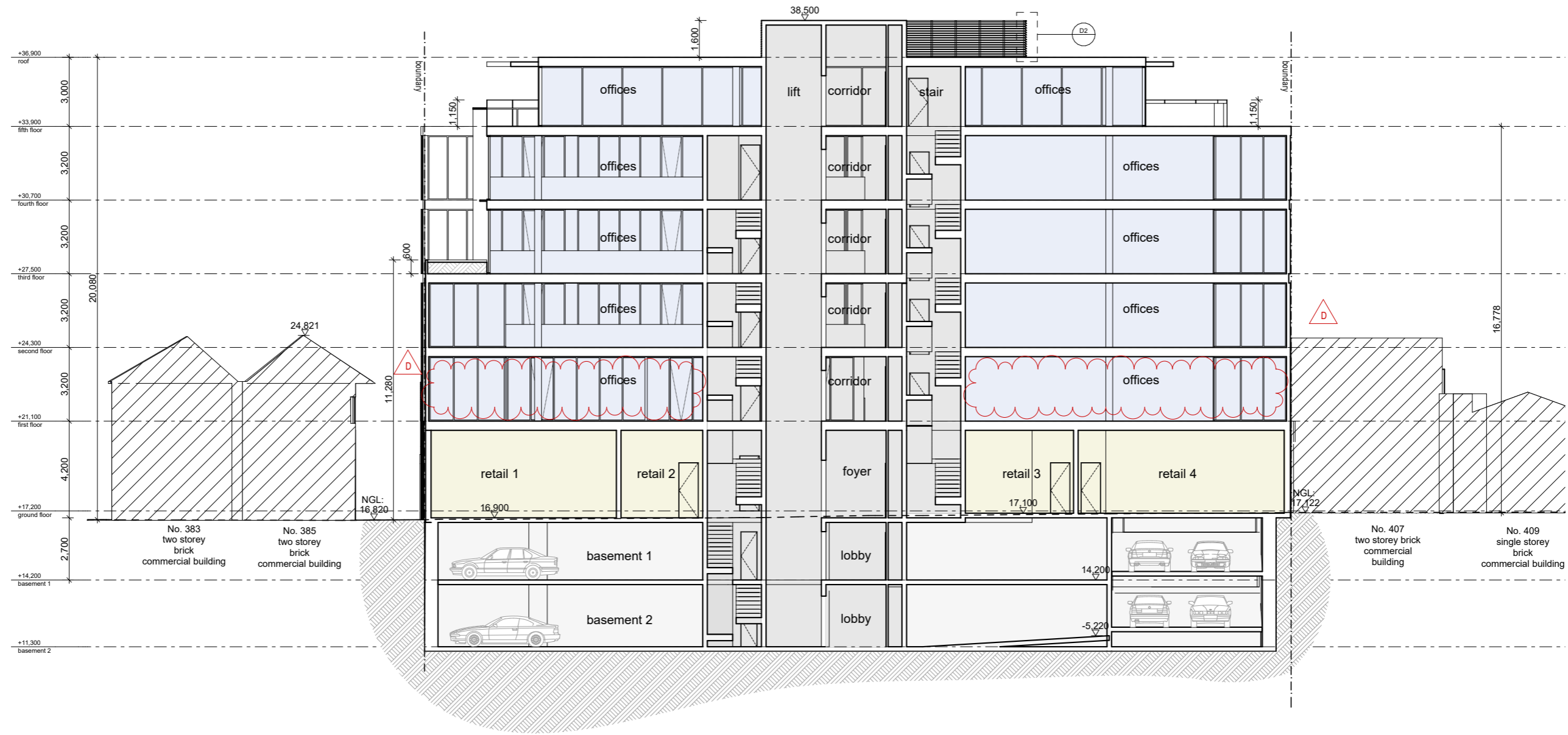
Section B - B scale 1:200
