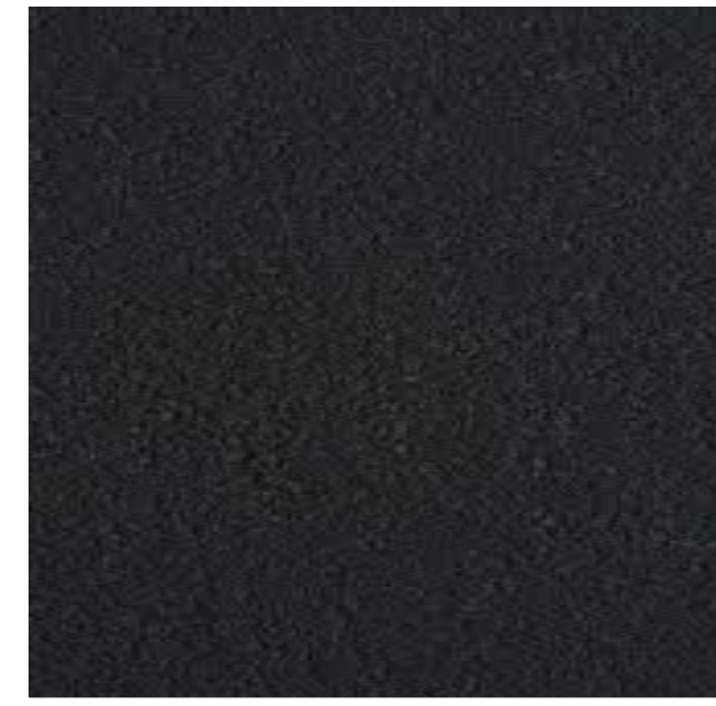
[CON.01] CONCRETE TYPE 02: CONCRETE FINISH - 'BLACK' SAND BLASTED
